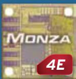
Monza 4E tag chips offer up to 496 bits of EPC memory, 128 bits of User memory, and a serialized TID to provide fast access to a larger memory, as well as meet the needs of applications requiring greater than 96 bit EPC numbers. Monza 4E also provides True3D antenna support.
