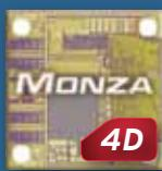
Monza 4D tag chips provide 128 bits of EPC memory, 32 bits of User memory, and a serialized TID. For applications where large memory is not required,
