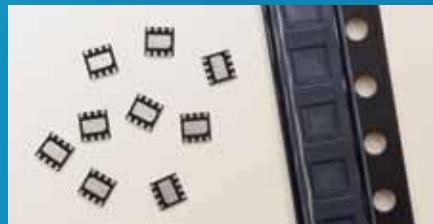
Monza 4 tag chips encapsulated in 8-pin µDFN packages accommodate surface-mount assembly and enable ruggedized tag designs.
