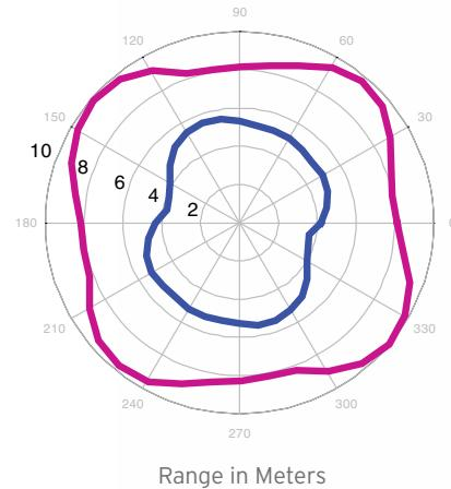
Monza 4 tag chip's True3D Antenna Technology removes blind spots and provides excellent read range
