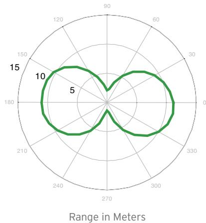
Tags based on conventional tag chips exhibit blind spots where read range drops significantly
