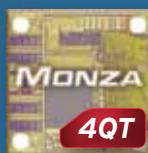
Monza 4QT tag chips offer 512 bits of user memory, 128 bits of EPC memory, block permlock capability, a serialized TID, and True3D antenna support. The extended User memory options support applications where users cannot count on a database connection. The 512 bits of User memory enables a portable, but private database to travel with the tag. Monza 4QT also provides Impinj's patent-pending QT™ technology, which protects data confidentiality and consumer privacy.
